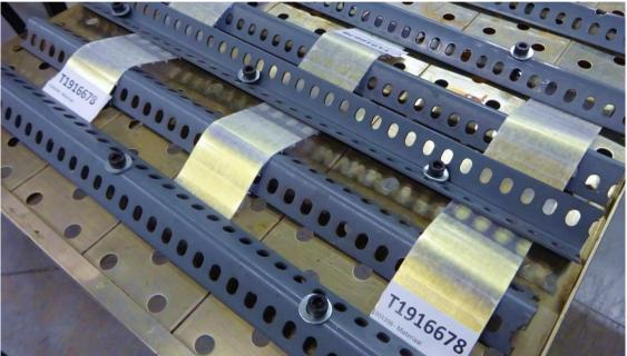
Figure 2: Clamping of the samples TOP-x5\_16mm
