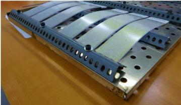
Figure 1: Clamping of the samples PC\_3mm en XT\_3mm
